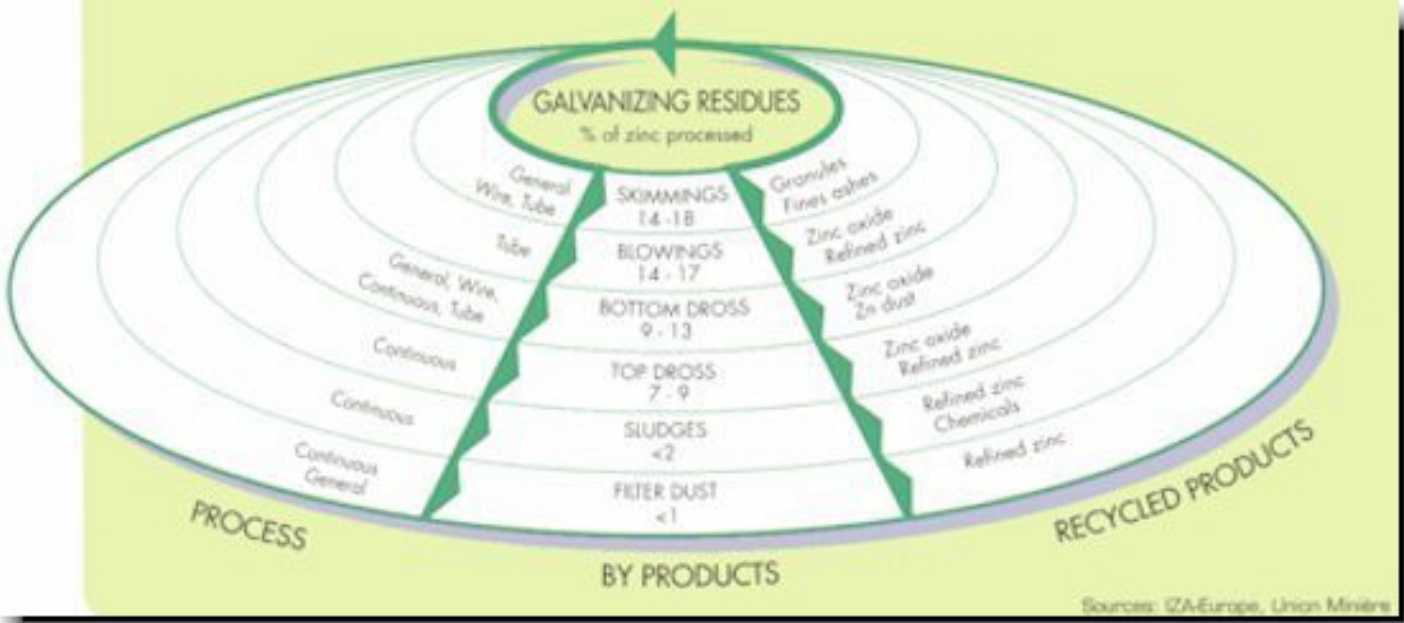
Figure 4 : Recycling of galvanizing process residues
